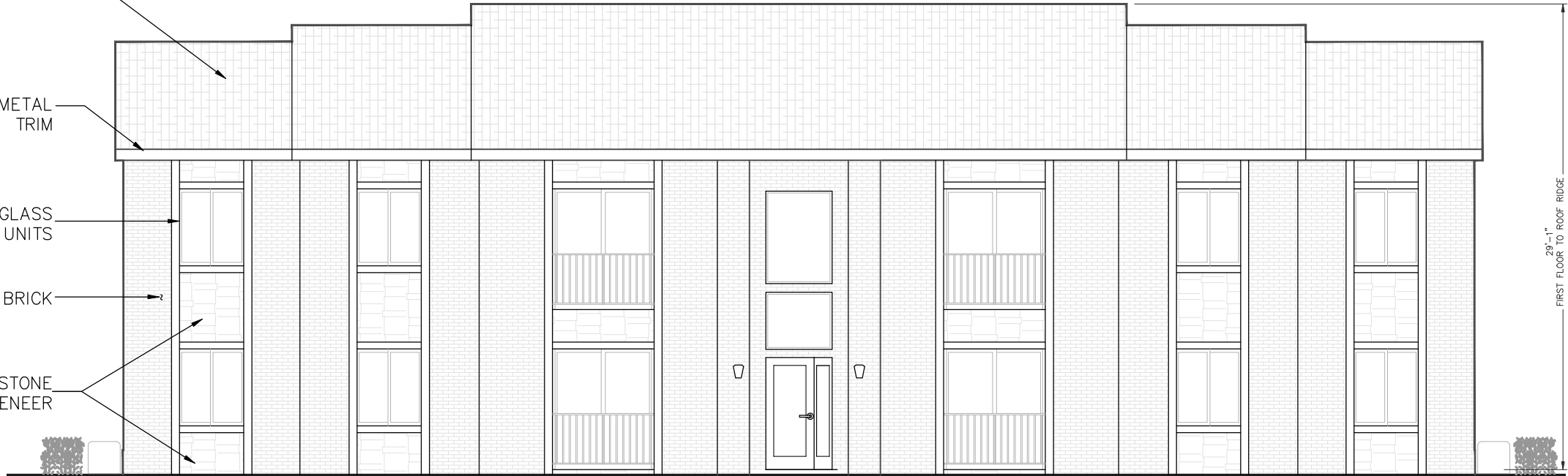
REAR ELEVATION (Bldgs 2 and 3)
