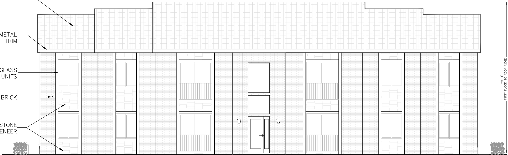
REAR ELEVATION (Bldgs 2 and 3)
