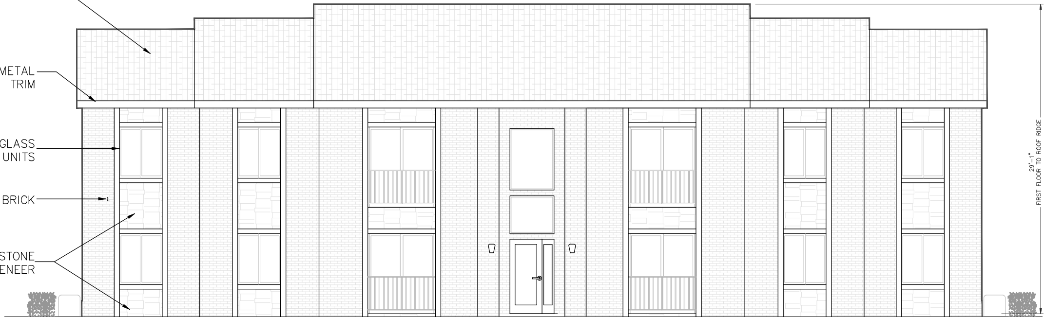
REAR ELEVATION (Bldgs 2 and 3)
