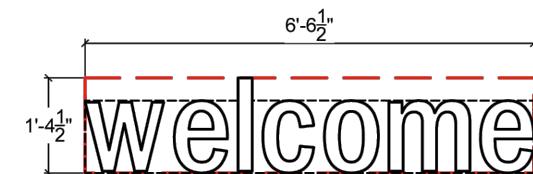
E5 WELCOME SIGN NTS NON-ILLUMINATED, DIE-CUT VINYL SURFACED APPLIED. CALCULATED 6.9 S.F. TOTAL 9.1 S.F.
