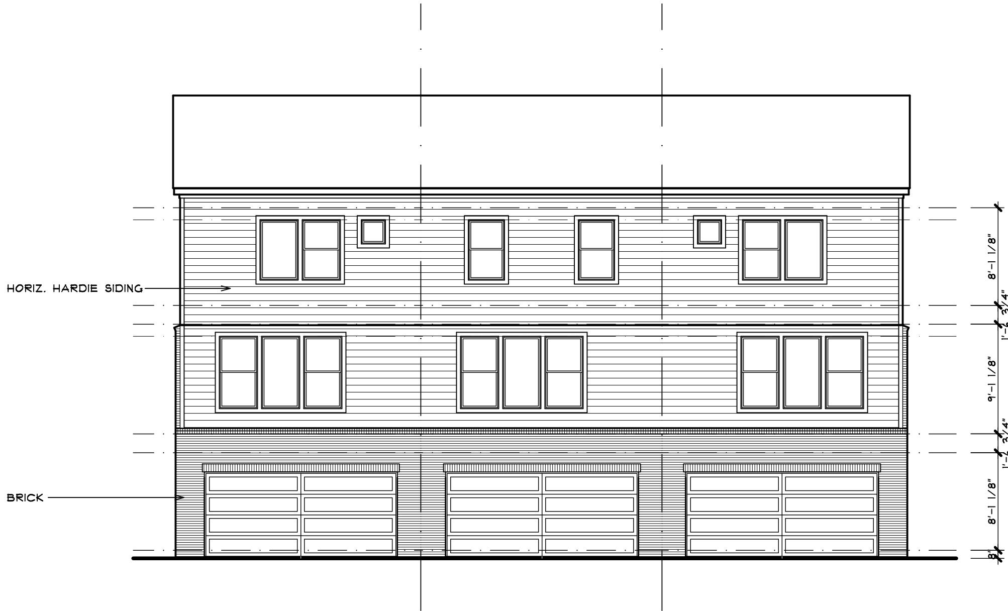
REAR ELEVATION 3 UNIT BUILDING
