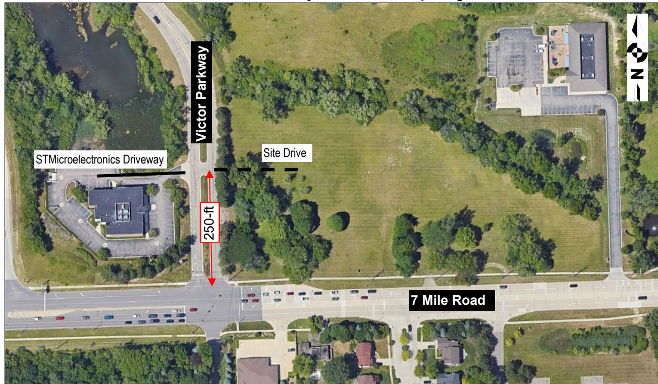
Exhibit 1: Driveway & Intersection Spacing
