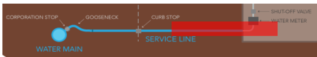
Figure 3: An example of a water service line
